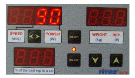
Further pressing of RESET opens the routine in which one can the limit for the sound signal (a double beet) that will occur after each repetition in which the power exceeds the limit. Power above this limit will be indicated by double beep. Setting 99% limit, the double beep will indicate the best value in current set. Setting 100 % limit disables this feature..
