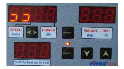
After transferring data from memory to the PC, CC (clear data) will show up on the display. For erasing memory you need to press buttons at the same time. If you return to the weight setting mode by pressing RESET data from previous set (sets) will remain the internal memory.
