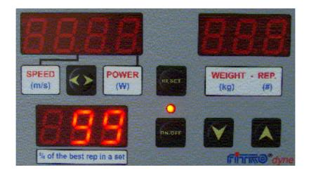
Further pressing of RESET opens the **SEND DATA** routine. To send data from the device's internal memory to your PC through interface one has to press , or enter the weight setting mode by pressing RESET button.
